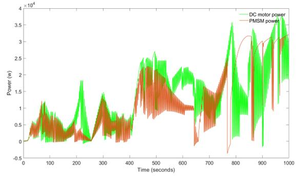
Fig. 17. Power consumption comparison of DC vs PMSM motors
