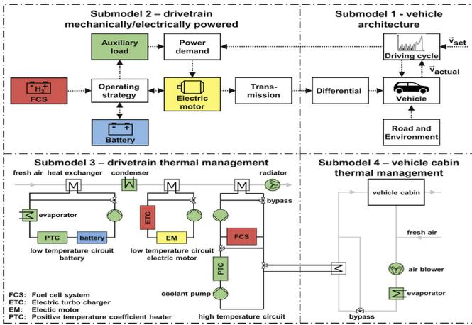
Fig. 1. Block diagram of an FCEV [18]
