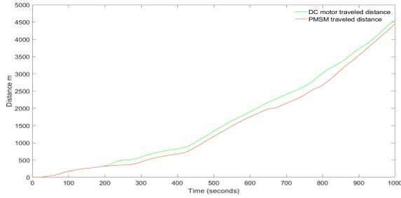
Fig. 19. Distance traveled - DC vs PMSM motors
