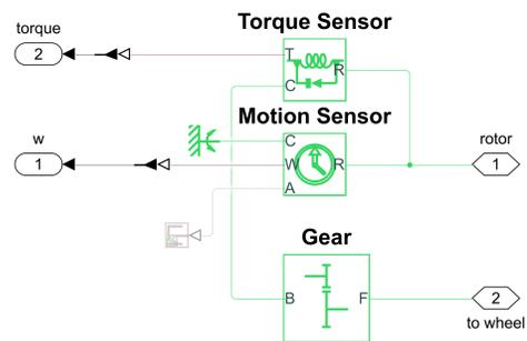
Fig. 7. Necessary sensors to measure the mechanical output of the designed vehicle
