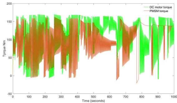
Fig. 16. Torque comparison of DC vs PMSM motors
