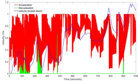
Fig. 12. Acceleration and deceleration of vehicle as per reference velocity
