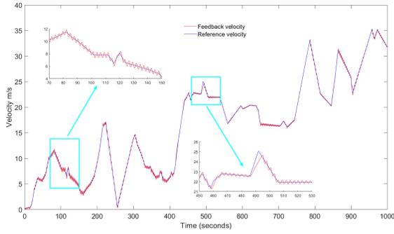
Fig. 14. Reference velocity vs actual velocity of the vehicle
