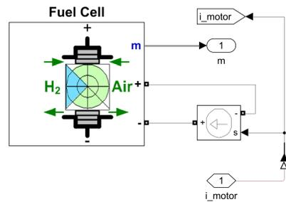
Fig. 6. Fuel cell model of the designed vehicle
