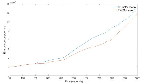
Fig. 18. Energy consumption comparison of DC vs PMSM motors
